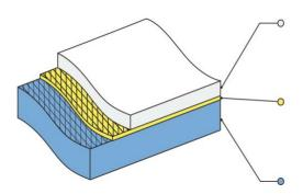
**Facestock:** 2 mil clear recycled polyester that offers excellent dimensional stability. The clear polyester provides high resolution imaging with excellent adhesion to UV curable inks.
